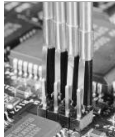
Probing with signal-ground pairs.
